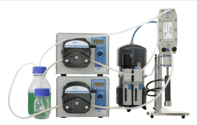
The Vibro-Lab35S membrane module is compatible with the Vibro-Lab35P and Vibro-LabEV drives
