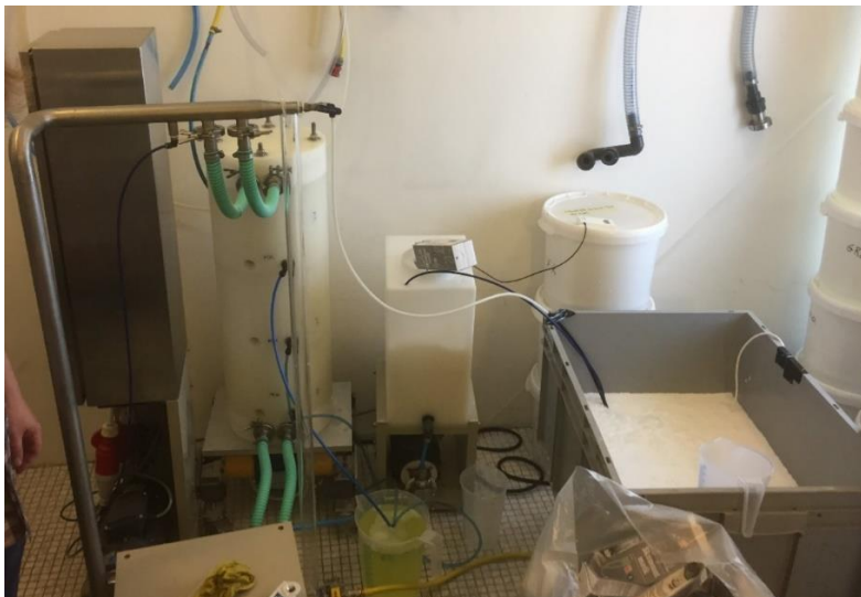
The 7,5 m 2 Vibro-I System during the Skim Milk concentration
